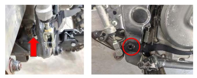
2. Remove the cotter pin, washer, and 8mm pin from the brake master cylinder.
