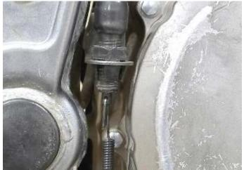
f. After adjusting the nut, re-start the Brake Light Switch Adjustment procedure.
