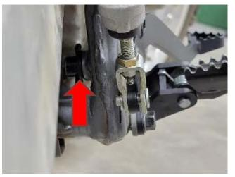
8. Reposition the brake master cylinder clevis over the brake lever. Reinstall the clevis pin and washer. Secure with the provided cotter pin.
