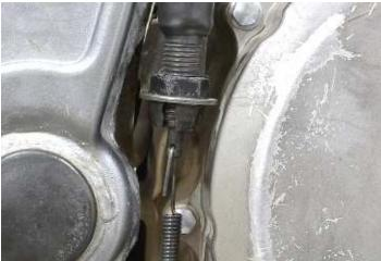
ii. If the plunger remains retracted after the foot brake lever is depressed, then the brake light switch adjuster nut needs to be adjusted down.
