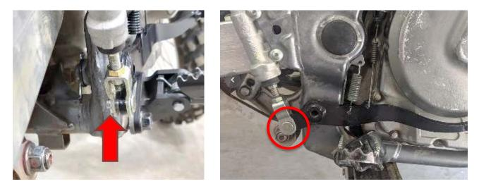
3. Carefully remove the brake lever by sliding the brake lever towards the right side of the motorcycle. Both the brake lever return spring and light switch spring can be left in place.
