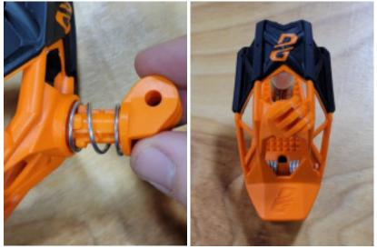
c. Position the C-clip next to the post. Use your thumb to press it into place on the pivot post.
