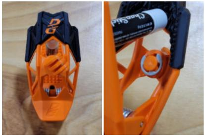
c. Remove C-clip with small flat blade screw driver.
