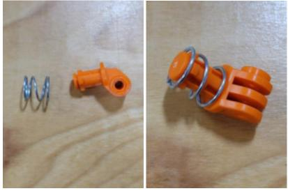
b. Insert pivot into gripper. Push and rotate to lock it in the compressed position.
